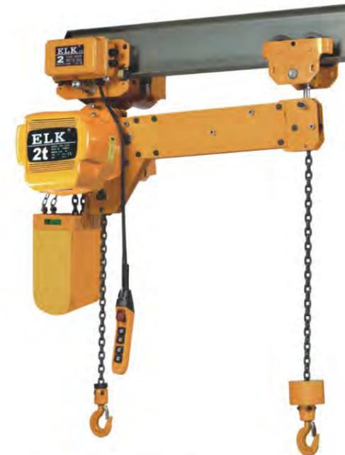
The hoist with dual hooks is equipped with a single motor but two hooks. It is widely applied for lifting long objects, or something which will rotate in operation. Two hooks can help to lift the object horizontally and safely. The distance between two hooks will be customized by your requirement.
